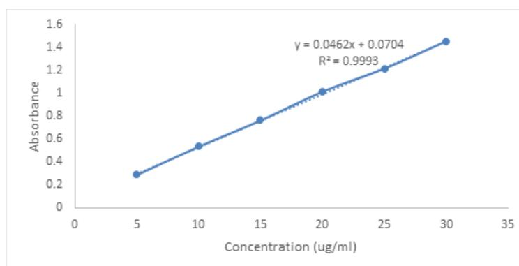
Figure 1. Calibration plot for acyclovir
